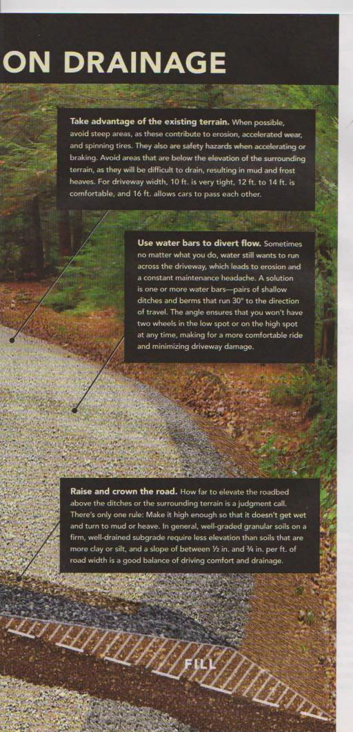
3-in.-minus gravel, which is a mixture of rocks sized from a maximum of 3 in. down to dust. In some cases, you might need to import all of the material for this layer.
